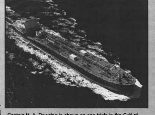
and a draft of 36 ft. (11 m). They will displace 50,035 long tons and have a DWT of 39,400.
