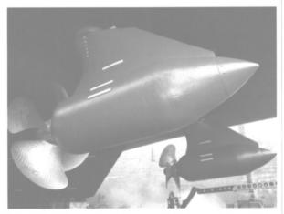
Millennium s Mermaid podded propellers were developed jointly by Alstom and Kamewa.
