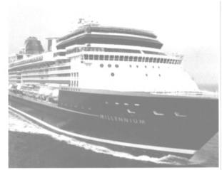
Measuring 965 ft. (294 m), Celebrity's Millennium is the first cruise vessel to house gas turbines.
