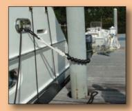
changes levels, removing the need to adjust mooring lines. TideMinders protect line up to one inch thick. The string of balls offers constant tension with built-in shock absorption.
