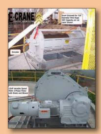
and a starting line pull of more than 40,000 lbs are the heart of this system. Each winch is driven by a 15 hp, 0 to 1,800 rpm, 460V - 3 Phase -60 Hz, inverter duty electric motor.
