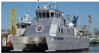
small ROV. The Apalachee structural design exceeds ABS high speed code for exposed routes and is USCG approved for 21 knots in 10 foot seas. The boat is outfitted with a custom 3000 pound capacity A-frame and trawl winch for over the stern operations. A Rapp Hydra Pro 5.5 mt knuckle boom crane on the port side is utilized for shore side transfer as well as offshore deployment of the Zodiac utility boat.
