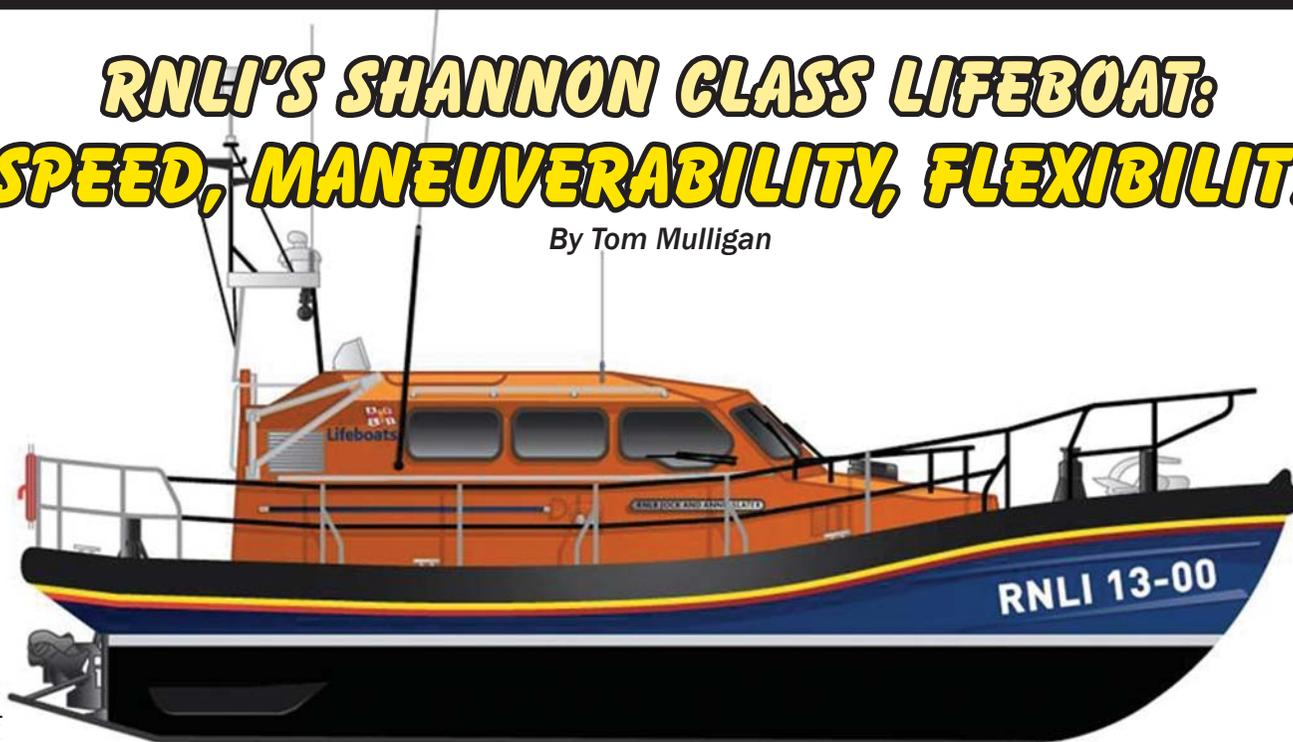
The latest lifeboat to join the fleet of the Royal National Lifeboat Institution, the main sea rescue service in the UK and Ireland, is the waterjet-propelled Shannon class, their most agile and maneuverable all-weather lifeboat yet to be deployed. Designed entirely in-house, cutting-edge technology has been used in this new boat to meet modern-day rescue service demands following the lead taken with the RNLI's introduction of the Shannon's sister lifeboat class, the Tamar, in 2005.
