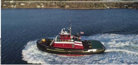
McAllister Towing has taken delivery of a newly built 6,770-horsepower shipdocking tug, Eileen McAllister, slated to enter service in Port Everglades, Fla. The 34th tractor tug in McAllister's fleet, Eileen McAllister was built by Washburn & Doughty in Maine and set sail for its new home port following delivery in April.
