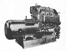
GENERAL MOTORS Diesel Generator Sets Model 3-268A, 152 BHP, 1200 RPM, heat ex-changer cooled, with 100 KW Generators, 450 volts AC, 3 phase, 60 cycles.
