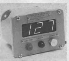
Propeller rpm indicator by Henschel.
