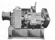
American Hoist and Derrick Company Winches with Westinghouse Motors, 50 HP, 230 Volts DC, complete with Contactor Panels, Master Switches, and Resistors. Type 66-single speed, single drum. Type 67-two speed, single drum.
