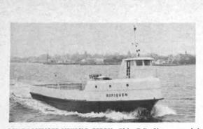
83' PASSENGER-VEHICLE FERRY. This T/L Class vessel is another in the line of Blount Botruc designs. She now operates in regular ferry service carrying 4 trailers and 50 passengers for the Commonwealth of Puerto Rico Ports Authority.
