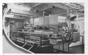
Steering gear was provided as a complete unit by Western Gear Corporation. It is operated by a Sperry system.
