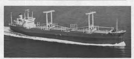
**NEW LUMBER CARRIER**—Mitsui Shipbuilding & Engineeering Co., Ltd., Japan, recently delivered at its Tamano Works the 19,000-dwt lumber carrier, Hiko Maru, to her owners, Sanko Steamship Co., Ltd. The 479-foot ship, which is to ply between Japan and North America, has three sets of 15-ton booms and one 20-ton boom, with strengthened upper deck, hatch coaming and hatch covers. The maximum trial speed of 18.59 knots was developed with the 9,400-bhp Mitsui B&W diesel engine.
