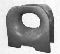
Clear opening 10" x 14" - 7" radius - with extended legs for welding to deck. Use as double or single bow chock. OAL 28" on base - OAW 14" - OAH 273/4" - Cast Steel.
