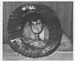
Shaped like a doughnut, this submarine was designed to catch herring efficiently in a net trailed behind the opening. **Paul White**, one of the University of Michigan students on the design team, looks through the opening to show where the trailing net is attached.
