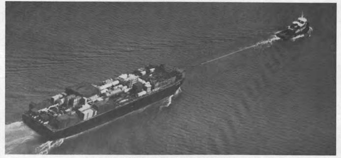
**1969** Hughes delivers pressure tank components, New Orleans to Maracaibo, Venezuela, on one of the world's largest deck cargo-carrying barges, towed by 4,000 BHP diesel tug.
