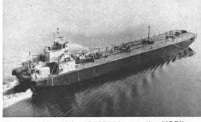
The 210' x 35' x 12'6", 10,800 bbls capacity, MOBIL TRADER is powered with M&T Harbormaster 466 h.p. F-7 drives.
