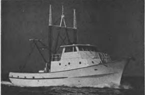
To meet the rising demand for durable and economical shrimp trawlers for long range operation, the Hatteras Yacht Division of North American Rockwell, Inc. has developed a standard 74foot molded fiberglass trawler. Production has started on this standard trawler in the firm's new New Bern, N.C. facility. The vessel was designed by J. B. Hargrave Naval Architects, Inc., West Palm Beach, Fla.
