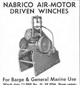
Winch duty 11,000 lbs. @ 39 FPM. Drum capac-ity 115 ft. of 1" wire. Drum size-11". Air motor mfg by Gardner-Denver-type MKB-A-reversible -11.5 HP @ 100 lbs. pressure. 1" Pipe con-nections for air. Units complete with air and hand brakes. Typical serial No. 458307. Just removed from ware and barres Good acception condition from unmanned barge. Good operating condition. 7 Units, with motors, available.
