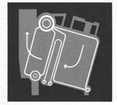
Schematic arrangement of a V2M-8 welded wall marine boiler. Boilers of this type are in fleet use aboard LKA class ships.
