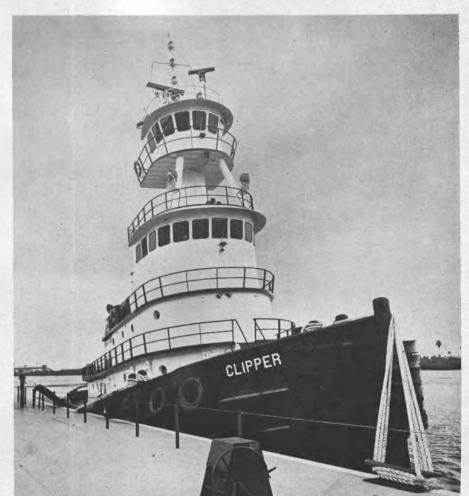
Tug Clipper features an elevated pilothouse-a unique installation on a seagoing tug
