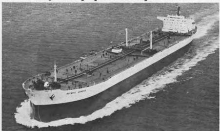
The Olympic Armour, first of five 216,000-dwt sisterships, is designed so that it can pass through the Suez Canal in ballast condition.
