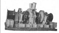
Below deck motor drive. Double Wildcat—driven by 50 HP—230 volt DC motor with vertical shaft and worm drive. Single speed—handles 7000 lb anchors and 60 fathoms of 15%" chain at 7 fathoms per minute. Wildcat centers 56". Complete with all controls and warping features. Total weight 27,500 lbs. With spares.
