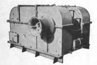
LAKESHORE UNWINCHES, with Allis-Chalmers Motors, 50 HP, 230 Volts DC, complete with Control Equipment.
