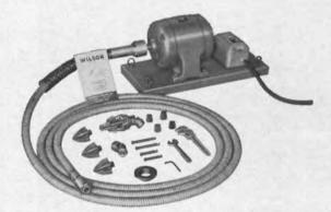
Electrically driven tube cleaner kits efficiently remove scale from 5/8"-4" OD straight tubes, 1"-4" OD curved tubes. Fast, thorough, safe.
