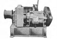
American Hoist and Derrick Company Winches with Westinghouse Motors, 50 HP, 230 Volts DC, complete with Contactor Panels, Master Switches, and Resistors. Type 66—single speed, single drum. Type 67—two speed, single drum.
