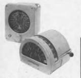
Henschel Engine-Order Telegraphs have been standard equipment since The Days of Steam. Current models are designed to be read conveniently from top or side. They lend themselves equally well to console or pedestal mounting. With today's trend to direct control from the bridge, we often furnish a combined throttle-telegraph lever unit.
