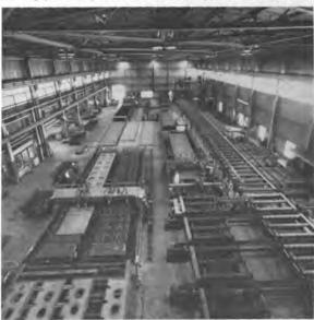
The fabrication building at Litton's Erie plant. Panels of 48-foot-long by 90-inch-wide plate with three stiffeners are produced on a production line in this building.
