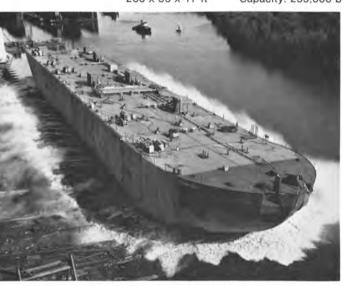
SEAGOING TANK BARGE 546 x 85 x 40 ft Capacity: 30,000 bbl
