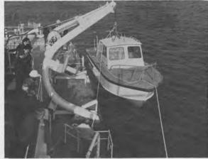
A 5,500-pound pilot launch is shown suspended on a single gantline from the "wishbone davit" aboard the New Jersey.
