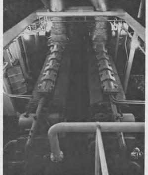
Starboard engine room showing two 3,500-hp General Motors Electro-Motive diesel engines.
