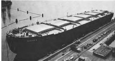
SEAGOING PHOSPHATE BARGE 420 x 80 x 37 ft Capacity: 664,025 cu ft
