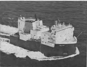
STUBBY, comprised of only bow and stern welded together, is shown leaving its birthplace at Litton's Ingalls Nuclear Shipbuilding yard in Pascagoula, Miss., to steam 2600 miles to Lake Erie, where the modular midbody was inserted to become the largest ore carrier on the lakes.
