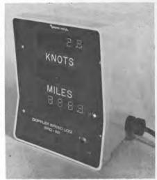
The doppler speed log provides an accurate measure of ship speed in water of any depth greater than 3 feet below the keel.
