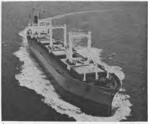
Approximate measurements of the Acritas are: 440 feet in length, 65 feet in breadth, 40 feet in depth, and a draft of 30 feet. Her main engine is a 5,130-bhp 1HI-S.E.M.T. Pielstick diesel engine and provides a service speed of 13.6 knots.
