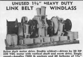
Below deck motor drive. Double wildcat—driven by 50 HP 230 VDC motor with vertical shoft and worm drive. Single speed—handles 7000 lb anchors and 60 fathoms of  $1\frac{5}{8}$ " chain at 7 fathoms per minute. Wildcat centers 56". Complete with all controls and warping features. Total weight 27 500 lbs. With spaces.
