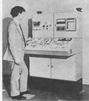
The control unit electronically records the main factors of performance, and the resulting charts are subsequently returned to Tank SAPP's Croydon offices where they are analyzed.
