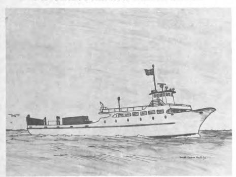
Artist's rendering of the vessel under way. With twin-diesel power, her 20-mph speed will enable her to make the 14-mile Orient Point-New London run in less than an hour.
