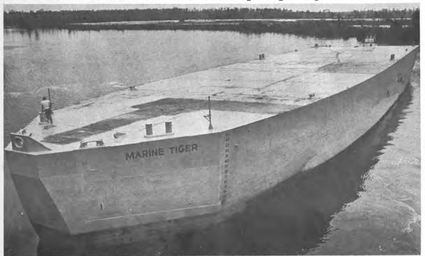
The midsection of the World War II troopship Marine Tiger was transformed into this sleek, white 300-foot namesake barge by Slocum Iron Works, Inc. The Marine Tiger and three sister barges will be used to service offshore rigs.
