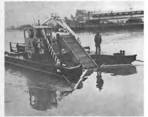
The forward throat area of the vessel incorporates a wideangle debris deflector leading into a conveyor. The throat area can also incorporate an oil skimmer attachment.
