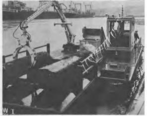
The hydraulic crane loader can lift sunken or floating objects from the throat area or from alongside the vessel and place the material on the aft deck.
