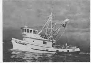
The Kimber is powered by a Detroit Diesel Model 12V71N delivering 350 continuous horsepower through a Twin Disc Model 514 reverse-reduction gear.
