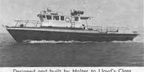
Designed and built by Halter to Lloyd's Class 100-A Nigerian Service classification, the new crewboat can accommodate 32 passengers.
