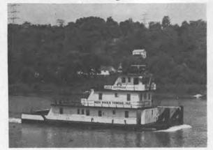
The M/V Leo D. Guttman, which provides living quarters for a crew of eight, has a pilothouse with an eye level of 24 feet.
