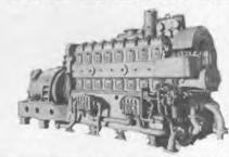
ENGINE: 8-268A—6½" bore x 7" stroke—1200 RPM—driving 200 KW Westinghouse generator—440 volts—3-phase—60 cycle—321 amps—80% power factor at 1200
