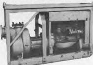
Reconditioned—mounted in portable steel frame, 1750 RPM—1100 GPM @ 100' head; 1500 GPM @ 70' head; 1800 GPM @ 20' head; 1800 GPM @ 20' head. Leroi gas engine—model D-201P3
