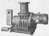
MOTOR: 10 HP—totally enclosed—fan cooled—continuous duty—horizontal flange mounted—special shaft & oil seal fitted—220/440/3/60—1760 RPM. CONTROL: Marine type watertight pushbutton—forward / reverse / stop—watertight starter box—rated for 40 starts/hour—triple pole contactor with silver contacts, thermal overload relay & trip adjustment. DIMENSIONS: Barrel 10" diam.—flange 10" diam.—approx. 26" wide & 36" long.
