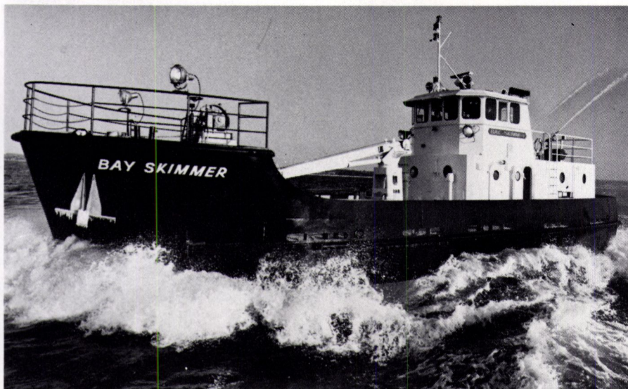
With its bow secured, the 100-ton Bay Skimmer cruises at better than 9 knots on Narragansett Bay. It carries a crane amidships to pick debris from its oil collection tank and to allow it to double as a general supply and patrol craft in Bantry Bay, Ireland.
