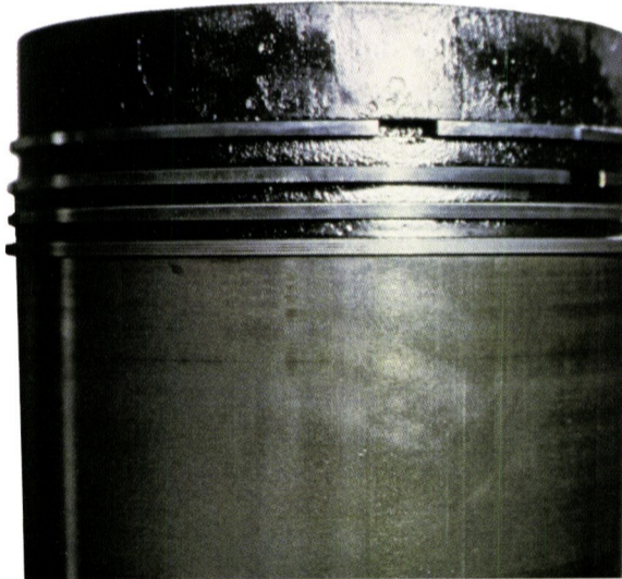
After over 23,000 hours, piston #1 of the starboard engine of an EMD 16-645 E7 shows light lacquer on skirt; rings in good condition, none stuck; only normal drag lines. Tornus Oil fights wear and lacquer buildup.
