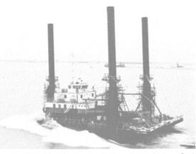
Self-propelled, jackup type well service barge Carl Fleming was launched recently at Singapore shipyard of Promet Private Limited. Positioning and emergency take-home power is provided by four GM diesels.
