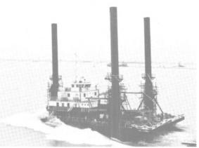
Self-propelled, jackup type well service barge Carl Fleming was launched recently at Singapore shipyard of Promet Private Limited. Positioning and emergency take-home power is provided by four GM diesels.
