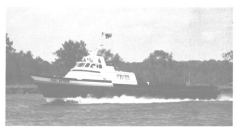
Crew/supply boat Port Arthur was completed recently by Progressive Shipbuilders & Fabricators, Inc. Built for Port Arthur, Inc., the all-aluminum vessel's four General Motors 12V71 diesels give her a top speed of 31 mph.
