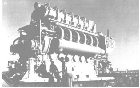
Two of these Enterprise RV-12 engines will power each of three bulk carriers under construction at Levingston yard.
