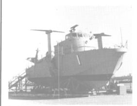
LENGTH: 74.4' OVERALL: BEAM: 21.4' EXTREME; DRAFT: MAX 4.5' SITTING 13.5' FOILS DOWN: DISPLACEMENT 56.8 FULL LOAD; CONDITION: VESSEL IS INCOMPLETE, PARTS AND ITEMS MISSING. THE PARAMETERS DESCRIBE THIS VESSEL WHEN IT WAS NEW, NOT AS IT IS NOW. VESSEL IS SOLD "AS IS, WHERE IS." WE URGE BIDDERS TO INCREPCT.
