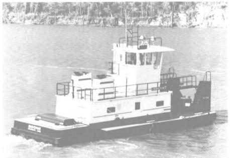
The M/V Boone, shown above, is powered by twin Caterpillar 3412 marine engines. The vessel, built by Dravo SteelShip, was recently delivered to Cincinnati Gas and Electric for use at their coal and lime facility on the Ohio River.
