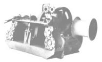
DRUM CAPACITY: 1250' of 1" wire in 9 layers or 2200' of 34" in 12 layers. Weight 11,300 lbs. DRUM DIMENSIONS: 22" diameter—20" between flanges; flange diameter 40"; two 16" gypsies. DRUM BRAKE: Contracting band type—asbestos lining—foot operated. WINCH DIMENSIONS: 12' long—8' wide—5' 10" high. Reconditioned by U.S. Navy. Equal to new.
