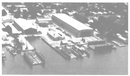
Conrad Industries, Inc., located along 450 feet of Atchafalaya River frontage in Morgan City, La., has expanded its facilities to triple production. A new metal building (right) measuring 360 by 100 by 45 feet houses new barge construction, new drydock construction, and is equipped with three 10-ton overhead cranes, and welding and plate-bending machines.
