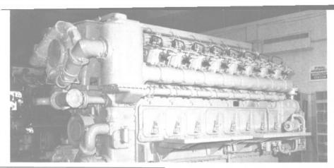
General Electric's turbocharged V-16 has rating of 3,500 bhp.
