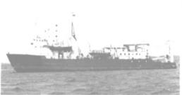
191' L.O.A.; 45' beam; 17' draft; 1349 G.R.T.; twin 2600 H.P. Main engines; bow thruster; heliport; accommodation 30; Ice classed; Deep water (6000') submersible if required; located West Coast.
