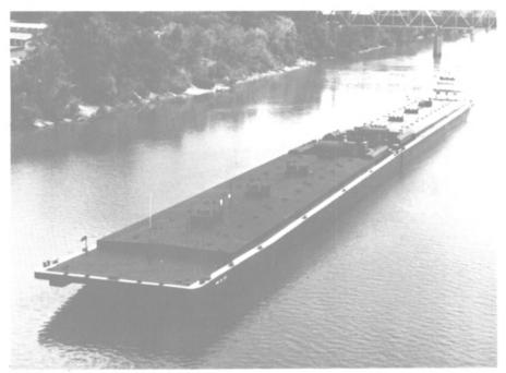
Second of two 297-foot barges built by Nashville Bridge Company (NABRICO) begins its journey to National Marine Service, Inc., St. Louis. The two double-skin, rake tank barges were specifically designed for asphalt service.
