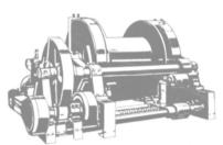
Heavy-duty Clyde with 36" diameter X 51" Face single drum. Flanges 68". CAPACITY: Up to 2800' of 2" wire rope. Normal line pull 40,000 lbs@ 50 FPM. Steam or air pressure required 125 to 250 PSI. Can be adapted to electric drive or increased steam or air pressure to a capacity of 82,000 lbs @ 20 FPM. Pawl holds 270,000 lb. pull from any layer. Equipped with level wind device. Approximate weight 30,000. DIMENSIONS: 12'6" wide—6'6" high. Write for details.
