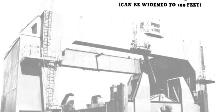
Originally Barge Handling. As used on LASH Ships. Manufactured by Alliance. Late Model built to ABS and MARAD requirements.
