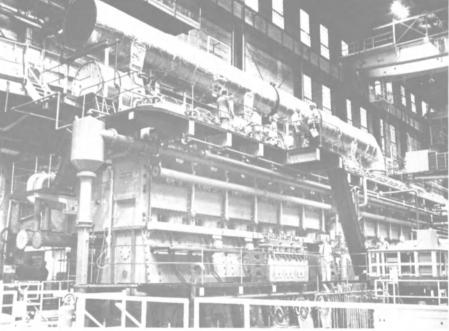
First Allis-Chalmers/Sulzer low-speed engine on test stand at A-C plant in Milwaukee.
