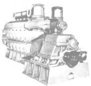
ENGINE: GM 12-567A-81/2X10-VEE type-2-cycle-747 RPM-electric starting-serial Nos. 1041 & 1060. GEAR: Falk Air Flex—reverse & reduction—2.48:1 forward— 2.52:1 reverse.
