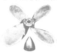
7' Diameter—pitch constant 4.699. Bore tapers from 6 1/8" to 4 53/64".  $14\frac{1}{2}"$  Taper equal to 1"/foot on diameter. U.S. Navy reconditioned. Average weight 1760 lbs.
