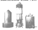
FOR EMERGENCY USE ON PASSENGER SHIPS, ETC. PUMP: JAS — 264 GPM — 171' head — two 6" inlets — one 5" outlet. MOTOR: 40 HP — 230 volts DC — 149 amps. COMPLETE WITH NASH — SELF PRIMING PUMP ATTACHED.
