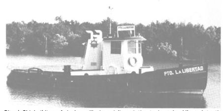
Diesel Shipbuilding of Jacksonville has delivered the tugboat La Libertad to the Port Authority of La Libertad, Ecuador. Boat is powered by two Detroit diesels.
