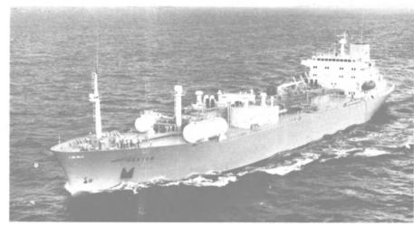
Versatile LPG/NH<sub>3</sub>/VCM tanker Hektor, completed recently by Moss Verft for A/S Nordsjogas, Stavanger, Norway, is powered by 14,400-bhp Horton/Sulzer diesel.
