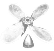
7' Diameter—pitch constant 4.699. Bore tapers from 6 1/8" to 4 53/64". 141/2" Taper equal to 1"/foot on diameter. U.S. Navy reconditioned. Average weight
