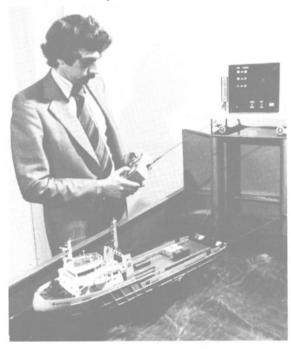
A new, unique mooring system that will keep a supply vessel permanently and safely moored to an oil rig at a pre-determined distance even in the worst sea conditions encountered in the North Sea is being developed in Scotland. A model of the Scomagg Hydraulics Ltd. system is shown above being tested in the company's factory at Bellshill, Lanarkshire.
