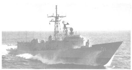
The HMAS Adelaide shown on sea trials on Puget Sound prior to recent delivery and commissioning. The General Electric gas-turbine-powered, guided-missile frigate is first of four being built by Todd Pacific Seattle for the Australian Navy.
