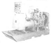
100 KW 440/220/3/60 generator driven by GM 4-71-T radiator cooled turbo charged diesel. P.F. 0.80—for T-2, etc. 1800 RPM. With switchgear. Generator is 10 wire—all voltages possible.
