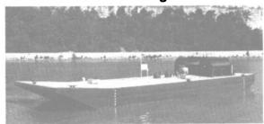
Riverway Shipyard Company, Grafton, III., recently completed construction of the KM-1, a new double-skin side, single-skin bottom raked barge (pictured above) for Kiesel Marine Service of St. Louis. The tank barge will be used as a midstreaming fuel barge for service in St. Louis.
