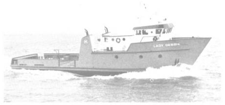
The recently delivered Lady Debbie (shown above) is the first of two twin-screw, 113-foot supply boats to be built by Bender Shipbuilding & Repair Company of Mobile for Keen Marine Services of Metairie, La. Constructed to a design of Maritime Engineering Services of Biloxi, Miss., the vessel is classed by the American Bureau of Shipping for Full Ocean Service, and meets U.S. Coast Guard Subchapter I requirements.
