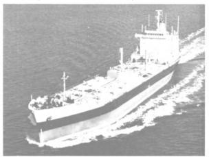
Similar to the two tankers for which Transamerica Delaval will provide main propulsion engines is this Falcon I-MSC vessel which entered service in 1975. Twin Delaval diesels power the original ships—a fleet of five. The two new tankers will be equipped with the same engines: Delaval "Enterprise" RV-16, mediumspeed diesels. Each 16-cylinder unit is rated at 7,360 bhp.
