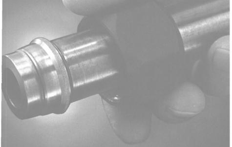
This ridge of metal illustrates how the Ferulok fitting forms a visible bite that allows each joint to be 100% inspected for proper make-up.
