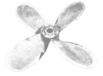
7' Diameter—pitch constant 4.699. Bore tapers from 6 1/8" to 4 53/64". 1412" Taper equal to 1"/foot on diameter. U.S. Navy reconditioned. Average weight 1760 lbs.
