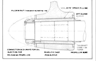
Elimination of key and keyway gets rid of stress concentrations, fretting corrosion \*Covered by world-wide patents
