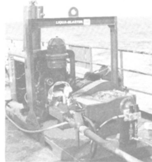
Diesel powered pump of a MARINE LIQUA-BLASTER onboard a vessel.
