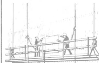
Platform for interior and exterior wall work.
