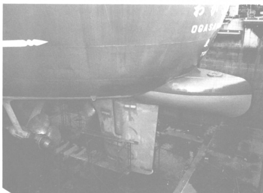
Kawasaki Stern End Bulb protrudes from center line of hull near full-load waterline. In test installation, this ship recorded five percent saving in propulsion.
