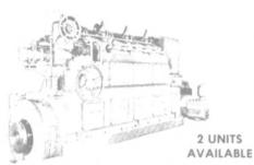
500 BHP @ 400 RPM. 4-Cylinder straight inline type -12½" X 16" — 2-stroke single acting — liquid cooled - direct reversible - CW rotation. With standard shaftconnected starting air compressor. 46,000 lbs., net weight-228" long-98" wide-132" high. Designed for heavy duty, rugged use, its extreme simplicity will result in lower operating and maintenance costs.
