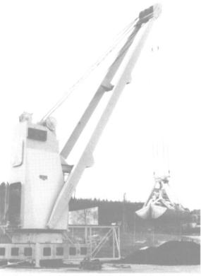
Hagglund's new 25-ton marine K-type crane showing its compact design and sheltered machinery
