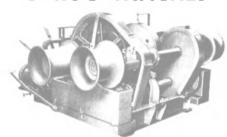
2-Speed — single drum — reverse throttle operation. LINE PULL: low gear 10,000 lbs — high gear 5,000. LINE SPEED: low gear 125 FPM based on 1st layer of 7/8" diam. rope — high gear 250 FPM based on 1st layer of 5/8" diam. rope. DRUM: 26" diam. — 20" long — 26" flange diam. Rope capacity of drum: 7/8" diam. rope in 6 layers — 650'; 5/8" diam: rope in 8 layers 1200'. Steam pressure at throttle 115 lbs. Operating weight 6450 lbs.
