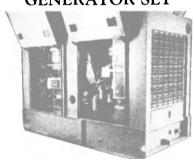
3-53 Detroit Diesel engine, Westinghouse Generator. 120/208 Volts, 3 phase, 60 Hz, 1800 RPM. With engine and generator control panel and circuit breaker. Skid mounted, radiator cooled. Sheet metal enclosure. 24 Volt starting. Built-in fuel tank. Reconnectible to: 240/416 - 440 V. Overall dimensions: 81"L., 55"H., 36"W. Freshly reconditioned, 2 hours of test time. Shipping Weight: 3,085 lbs.
