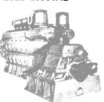
ENGINE: GM 12-567A-8½ X 10-V-type-2-cycle-747 RPM - electric starting. GEAR: Falk AirFlex - reverse & reduction - 2.48:1 forward - 2.52:1 reverse.
