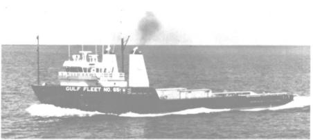
Gulf Fleet Marine's towing/supply vessel powered by GM EMD12-645 E7C main, and DD 12V-71 bow-thruster engines.
