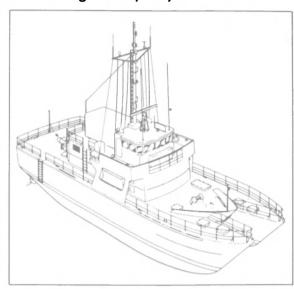
Minehunter features catamaran hull, fiberglass and foam sandwich construction, and weapons systems by Krupp Atlas Electronik.
