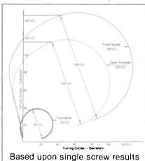
Towmaster's triple rudders create flow variations on themselves—a cascade effect—which permits 60° helm angles before rudder stall occurs. The result is impressive. Research documents that when a Towmaster System is compared with fixed nozzle and open propeller systems, turning diameters are routinely reduced by 90% and 65%, respectively.
