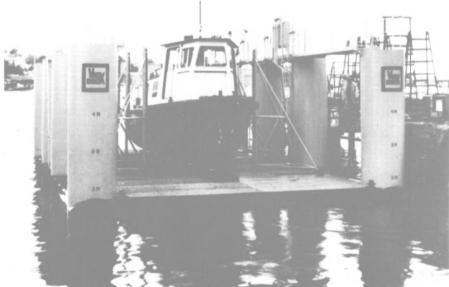
Unique floating drydock that uses compressed air to blow water from its ballast tanks will be built by companies in the U.S. and Canada.
