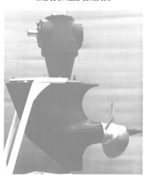
Strut drives up to 3,000 horsepower have been built by Maritime Industries.
