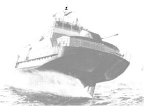
A patrol hydrofoil version of the Boeing Jetfoil for which Indonesia has signed a cooperative manufacturing agreement with Boeing Marine Systems.
