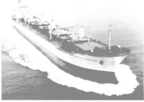
Designed as the largest bulk carrier that can transit the Panama Canal the Maersk Seragoon features a bulb stern and
