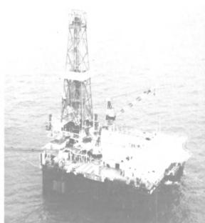
Sedco 602 rig has main deck 170 by 170 feet and can drill to 20,000 feet in water depths from 25 to 180 feet. Living quarters for crew of 88 include hospital and recreation room. national drilling contractors, operating a fleet of more than 40 offshore units around the world. Occidental Exploration and Production, established for 22 years, is well known in the field of oil exploration, production, and refining.
