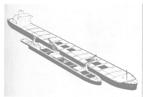
Coal topping off barge built by Bay Shipbuilding utilizes two 25-ton cranes to transfer 1,500tons of coal per hour.
