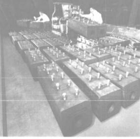
Components of an extruded EPDM/butyl fendering system receive the final inspection at the Uniroyal Engineered Systems plant in Mishawaka, Ind., prior to shipping to the ARAMCO maritime company for use on one of its 6,000-bhp Water Tractor tugboats.
