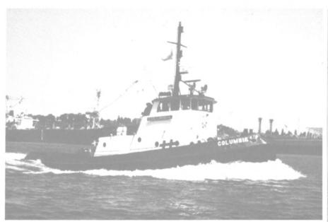
The 96-foot tug Columbia shown above was doubled in horsepower with the installation of two new 1,270-hp Stork-Werkspoor engines.
