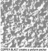
COPPER BLAST creates a uniform ancho pattern which provides good coating adhesion.
