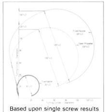
Together, they create a cascade effect that can allow 60° helm angles before rudder stall occurs.
