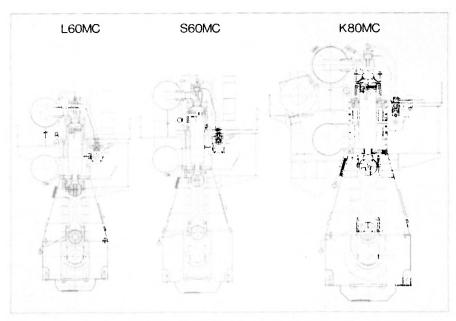
Cross-section drawings of K, L and S-MC engines. Courtesy of M.A.N.-B&W Diesel A/S
