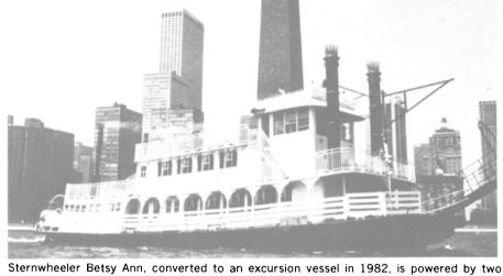
Hagglund hydraulic motors driven by hydraulic pumps/diesel engines.
