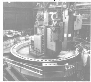
MAN GHH's portable large-capacity machining facility can be disassembled for transport.
