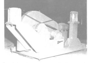
New Rightway ERP Long Distance Car Puller features frame-mounted sheaves for added control and economy.
