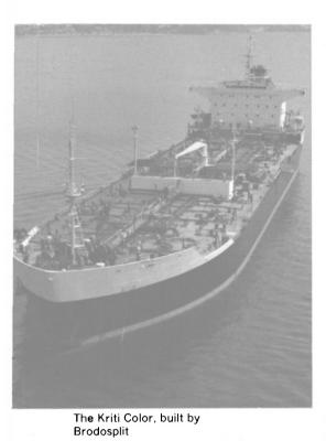
The vessel is classified +1A1, General Cargo/Container/Car Carrier, RO/RO, EO by Det norske Veritas.
