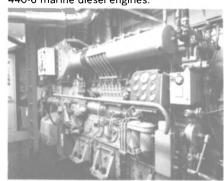
The TBD 440-6 marine diesel engine, rated at 979 hp at 900 rpm, installed aboard the African tug Djoliba.
