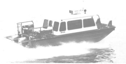
MonArk's new 26-foot survey boat is powered by two Outboard Marine Corp. "sea drives" rated each at 155 hp, yielding a top speed of approximately 32 knots.
