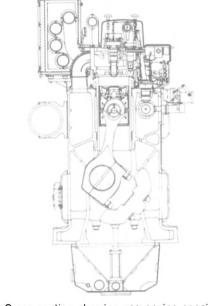
Cross section showing gas engine specific equipment added to a standard Vasa 32 diesel engine.
