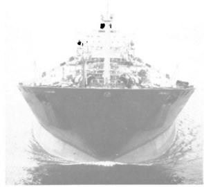
The M/T Chrisholm has a double skin and double deck that contribute to safety as well as insulating the cargo against thermal loss and overheating from the sun.
