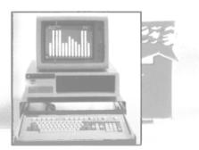
**OCEAN MOTIONS -**Ship Loading Computers For measuring and monitoring stress while handling cargo. User Friendly • All calculations performed for the ship in any condition or combination of conditions, including: her Intact. grounded... damaged... or flooded • Six (6) canned loading conditions pre-programmed for instant retrieval • All IBM hardware "marinized" and approved by ABS, LRS, and BV; plus software approvals from all agencies.
