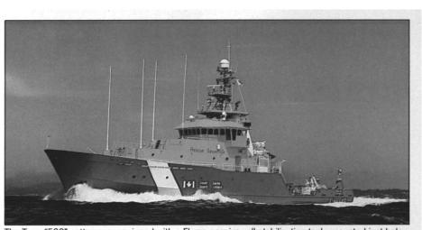
The Type "500" cutters are equipped with a Flume passive roll stabilization tank, mounted just below and forward of the bridge to significantly reduce roll amplitude in the severe weather conditions in which the cutters must operate. Maneuverability is aided by a 500-hp tunnel-type bow thruster.
