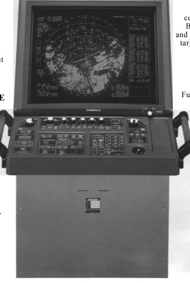
On-screen data readouts include range, bearing, course, speed, CPA, TCPA, BCR (bow crossing range), and BCT for up to 3 selected targets, as well as own ship course and speed.
