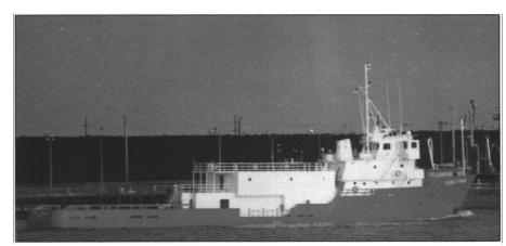
The Veesea Typhoon has been rebuilt to ABS standards, Maltese Cross A-I hull, equipment and AMS machinery, ABS International Loadline and USCG OSV certification.
