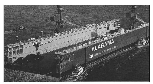
The ALABAMA has a lifting capacity of 225,000 DWT or 40,000 tons displacement. • Normal maximum draft over six-foot keel blocks is 32 feet.
