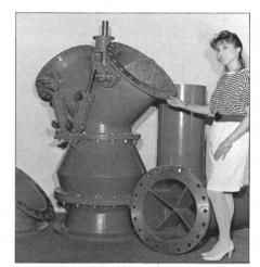
Omnithruster RPV 575-A Gamma series rated at 250 hp DC motor drive, Canadian Coast Guard, Navaids vessel Provo Wallis.
