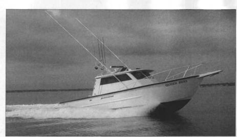
The offshore research craft Queen Bess is a new model deep vee welded aluminum boat developed by Thomas Marine Inc.
