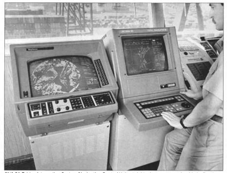
SNA-91 Bridge Integration System Navigation Control Unit, at right, shown at console with the Raytheon Pathfinder/ST ARPA. The SNA-91 computerized system presents a total ship management picture at a glance, including: engine, hull, weather, autopilot, and navigation information.
