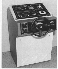
A sliding drawer inside the Nautamaster steering control stand allows mounting of the Polaris MK2 gyrocompass, thus providing easy access for maintenance and service operations; incorporated in the upper steering console plate of the Nautamaster is the control panel of the gyrocompass equipment.
