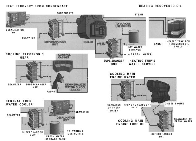
Naval ships, fleet oilers, commercial containerships, tankers and dredges are successfully finding new ways to operate more efficiently at lower cost, by utilizing Tranter's unsurpassed plate-type heat exchanger technology. Schematics presented here illustrate typical ways they are doing it.
