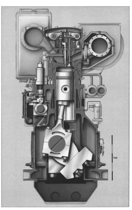
Cross-sectional drawing of the L58/64 diesel from MAN B&W's medium-speed engine family.
