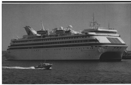
The first of her kind, the SSC Radisson Diamond utilizes SWATH technology in order to offer a large stable platform, while minimizing propulsion noise and vibration.
