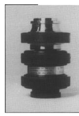
**ER12 End Fittings** and Hose: Qualified Under Military Specification MIL-H-24136/1 Products include 5, 6, and 8 inch bronze hose end fittings and synthetic rubber hose utilized in shipboard fresh water, salt water, fuel, and oil systems. End fitting configurations include straight and 90 degree flange ends, split clamp ends. and hose doglegs.
