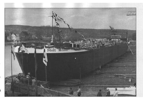
The M/T Stolt Mosel, built by Bayerische Schiffbau GmbH shipyard in Erlenbach, Germany, is one of five 2,100-dwt inland chemical I tankers designed by Stolt-Nielsen to transport bulk liquid along the Rhine .
