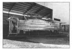
The deck structure of the Swath vessel Navatek II, which will be used as an excursion boat off the Hawaiian Islands, was built in a high bay building at the Seattle shipyard Workboats Northwest. The overall structure, while stout enough to carry passengers at sea, weighed only 16,000 pounds when shipped.
