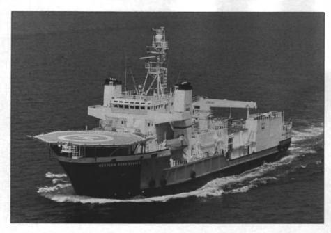
The Western Renaissance, reportedly the world's largest and most advanced well stimulation vessel, was christened by The Western Company of North America. The 308-foot ship was designed and built to provide proppant fracturing, acid fracturing, matrix acidizing and nitrogen services in the North Sea.
