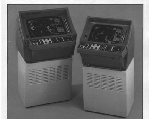
PATHFINDER/ST ARPA: 34-cm or 25-cm PPIs (16" or 12" diagonal CRT IMO equivalents) provide automatic tracking of up to 40 targets with vectors and readouts for the most dangerous 20. Have auto and manual acquisition, and unique trial maneuvers. PATHFINDER/ST TM/EP: 34-cm or 25-cm PPIs (16" or 12" diagonal CRT IMO equivalents) have True and Relative Motion displays. Electronic Plotting, course, speed, bearing, range, CPA, and TCPA for two selected targets.
