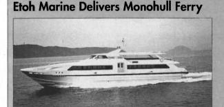
Etoh Marine Corp., Imari City, Japan, deliv-ered the *Fuki 8*, a 235-passenger monohull ves-sel, earlier this year for operation between Tomishima and Akashi, Japan. The ferry is 110 feet (33.5 m) long, with a beam of 21 feet (6.5 m) and a draft of three feet (1 m).
