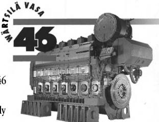
The Wartsila Vasa 46 engine has an output range of 3,620 to 17,550 kW.
