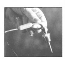
TERMOCOUPLE temperature sensors check exhaust ports on each cylinder of the Detroit Diesel, and two measure raw water and engine coolant. All sensor leads are routed to a junction box, then to the pilot house.
