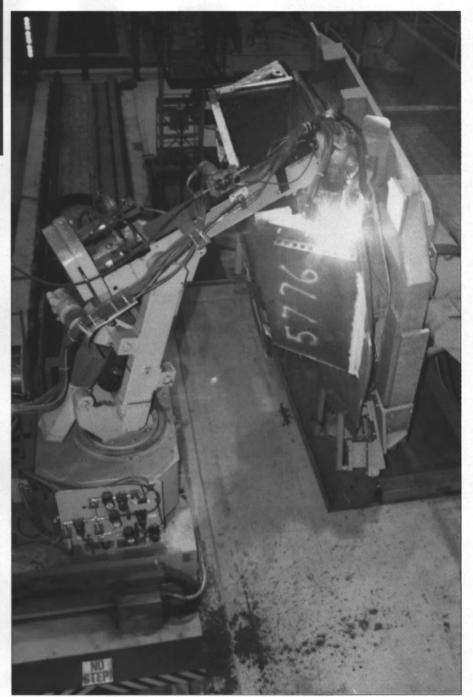
CYBO Robots helped modernize General Dynamics' Land Systems Div.'s Lima, Ohio plant with robotic welding stations to build the M1A1 Abrams battle tanks more efficiently. The company is currently working—with the help of the government and shipbuilders—to develop portable shipbuilding robotics to help make the U.S. competitive on an international level.
