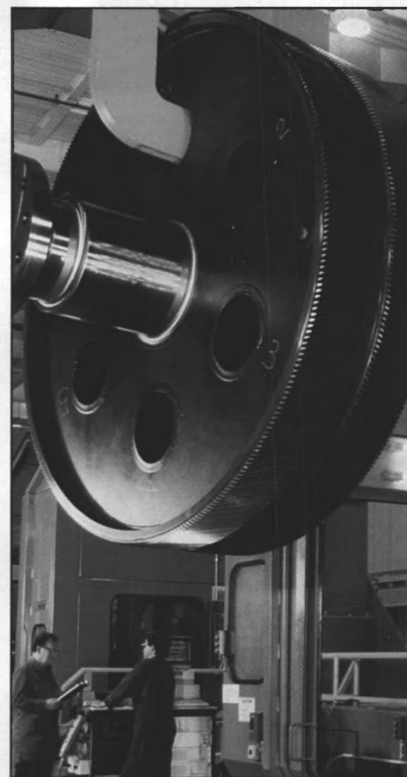
An advanced grinding machine finishes the teeth on GE gears to tolerances which can not be seen by the human eye. GE's world-class facility in Lynn, Mass., is dedicated to the design, manufacture and test of propulsion gears for the U.S. Navy and commercial ships such as LNG tankers, the Arleigh-Burke DDG-51 destroyers and NASSCO-built Sealift ships.
