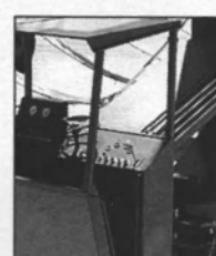
Closed circuit TV, digital readouts and a powered 'swing' operator's compartment to ease operations.
