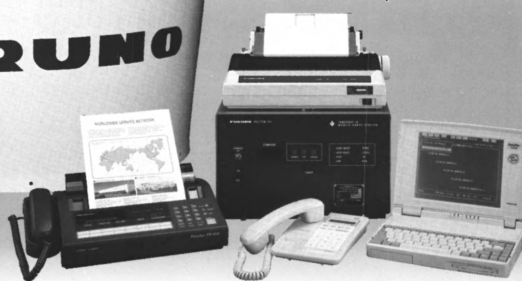
Furuno's Felcom 80 Satcom-B Vessel Communications System
