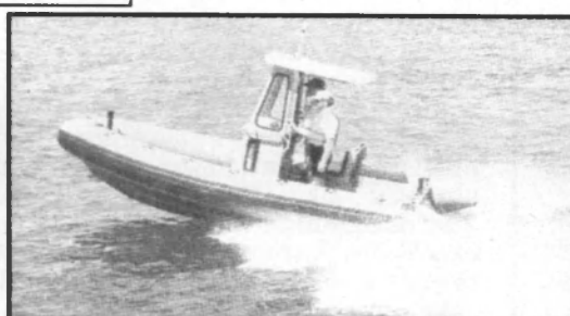
ZODIAC HURRICANE 560 Smallest RHI boat with inboard power. Available in gas or diesel with jet or outdrive
