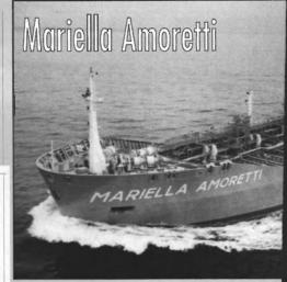
with the following class notation: RINA \*100 A 1.1, Nav IL, MN Cst (OIL/CHEM), ESP IAQ1, IAI, IAP, SC, PMS, P, NAU (OMBO), APS, IWS, TMS, MAN, IIQ, IV, EP2.
