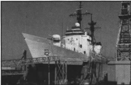
Bellingham Bay Shipyard recently completed a pair of U.S. Coast Guard repair contracts worth \$2.8 million for the 378 ft. (115 m) cutters Mellon and Midgett. In addition to maintenance and voyage repair work, both projects involved drydocking, complete blasting and painting of freeboard and underwater body, rudder bearing replacements, and cooler and piping renewals on the ships' supplementary gas turbine engines.
