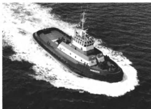
The tractor tug NAMAHOE, now in service in Hawaii; 4,400 HP with twin Z-drives: 105' x 34' x 16.5' (32 x 10.4 x 5m).
