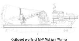
is equipped to provide offshore flowline installation, offshore umbilical installation and subsea construction. With 3-3,000-hp azimuthing thrusters on the stern and 2-2,000-hp tunnel thrusters in the bow, the vessel is also able to provide worldwide operations.
