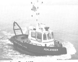
Damen Stan Tug 1405 Twin-Screw conventional tug with propeller no22tes
