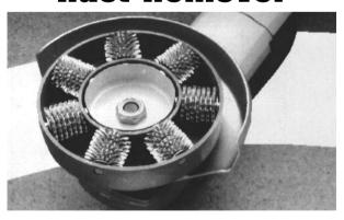
Rapidly remove paint, rust, scale, barnacles, and other hard coatings from metal and concrete surfaces without heavy pressure. New Swirl-Off scarifier attaches to your grinder, sander, drill, or polisher. Rotary tool scours tough deposits. Using pneumatic tools, it removes marine growths underwater. Easier, faster, and safer than scraping, sandblasting, or chemicals. There's nothing else like it! Ask for Bulletin MAR-1 showing many models and styles.
