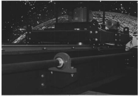
Craft Bearing used its Split Roller Bearing to tui an ordinary pipe into a precision drive shaft.
