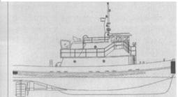
The tug will be powered by twin main engines producing 1,710 hp. Since the tug will be involved in operations in low bridge clearance areas, its superstructure and mast were modified to a low profile to meet a 19 ft. air gap clearance. Also onboard will be a hydraulically-operated stern towing winch to increase the vessel's capabilities and versatility.
