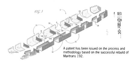
vative double hulling of an existing single hull barge, an internal double hull rebuild which was patented in 1999. To date, Maritrans reports that Maritrans 192 and Maritrans 244 are rebuilt and operating flawlessly, while Maritrans 252 recently joined the
