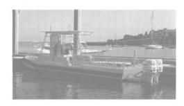
26/28 Center Console delivered to US.Navy. Options include: removable top, soft sides & dive tank holders. Twin 150 Evinrudes w/48mph top speed.
