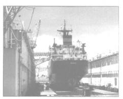
18,000 Tons with 12" freeboard at low point of pontoon deck
