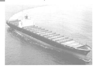
Constructed by Samsung Heavy Industries, the 983-ft. (299.8-m), 6,200-teu containership owned by NYK is an example of the new, larger, more efficient containerships.
