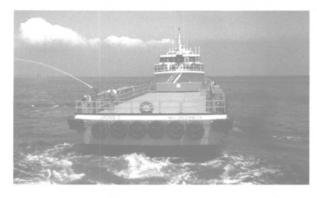
A. K. Suda, Inc. was approached by LaForce Shipyard of Bayou LaBatre, Ala. to design a crew/supply boat that would be faster, carry more deck load and more passengers and still be delivered at an economical price. The result is the 160 x 32-ft. (48.7 x 9.7-m) high-speed crew/supply boat that was recently delivered by LaForce at their Alabama yard.
