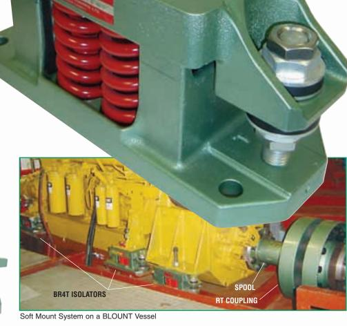
The Lo-Rez Soft Mount® System uses BR4T Isolators and the RT Steel-Bolted Rubber Coupling to mechanically and acoustically isolate the engine and gearbox from the hull and shaft line. There is no metal-to-metal contact within the BR4T Isolator or within the RT Coupling. Additionally, propellor thrust pulsations are absorbed by the coupling and isolators. Over 450 applications of these systems exist.
