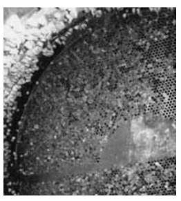
Typical fouled condensor tube plate.
