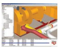
New collision detection and management system in Tribon M3 Service Pack 3. The two pipe flanges connecting to the mooring winch collide and this is reported in the list window in the lower part of the screen.
