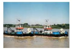
sels will be deployed in the Caspian Sea on a long term contract, supporting the local oil- and gas industry. Because of the local conditions the draft is limited to one meter and despite this limited draft, the vessels have a bollard pull in excess of 9 tons.
