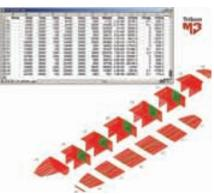
Result of preliminary block splitting in Tribon M3 Service Pack 3. Report file showing weights and COGs (Center of Gravity) for a preliminary hull block definition.
