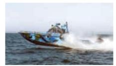
waterway security. The Mongoose series of FPB vessels, ranging from 25-120 ft. (7.6-36.6m) are built with Ceramic Reinforced Plastics (CRP). Mongoose MK-1 is a 27-ft. (8.2 m) high-speed mono-hull vessel, designed to provide maximum control at both
