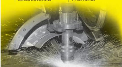
ESAB's unique integration of cutting machine, control and plasma flow control has created a new era in plasma cutting and beveling. The Expert Motion Plasma Variable Bevel Angle (VBA) System is the most accurate and easy-to-use beveling system in the industry. The reduced size and weight allows its use on smaller machines or as a retrofit, making beveling more affordable. Ask for ESAB by name.
