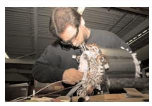
A technician inserts coils into the stator of an AC motor.
