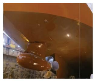
Designed by Aker Arctic Technology, assembled in Helsinki with the hull from German Aker Ostsee, Norilskiy Nickel is the first double-acting cargo vessel newbuilding for Arctic operation. The ship is fitted with two 13 MW Azipod units supplied by ABB.
