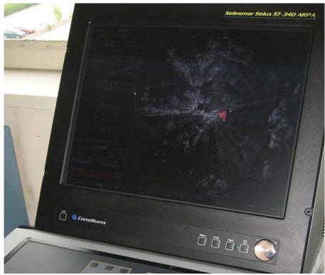
An oil slick detection radar system by Consilium of type Selesmar SeluxST was also installed.
