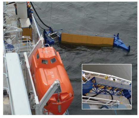
The vessel has one pair of Lamor's rigid 12m sweeping arms, each unit with an exchangeable weir skimmer module and brush module. INSET: When not in use, the sweeping armes are stored on the aft deck.
