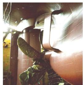
**Typical Stern-Appended** Hydrodynamic Energy Saving Devices (ESD) applicable for single-screw, high block coefficient ships such as tankers and bulkers. (The first photo is a Propeller Cap Turbine (PCT) retro-fitted on a tanker which had been constructed with a Wake Equalizing Duct (WED). The second photo shows a chemical carrier under construction with the Simplified Compensative Nozzle (SCN) being installed.)
