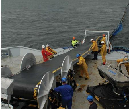
The heavy duty oil boom is stored in 125m lengths on own reels.
