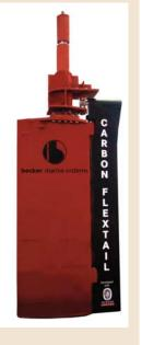
properties such as a slim design provides less drag and improved lift. Composite rudder flaps are available for all types of Becker high-efficiency rudders such as FKSR, SA/SC and Heracles rudders. Becker also offers composite material for rudder stocks. The weight of a rudder stock for a 8,400 TEU container ship, for example, can be reduced from 72.2t to 26.6t by using the new material.
