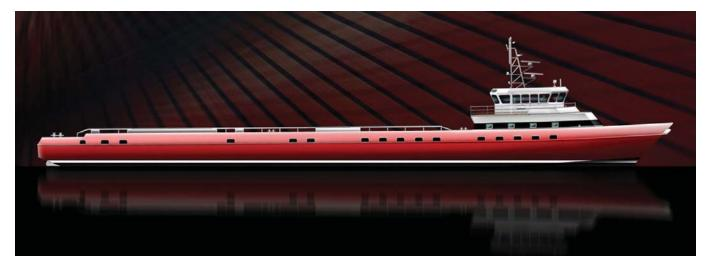
Incat Crowther has set its sights on the title of the world's largest ever Fast Supply Vessel, as it has been contracted to assist with the design of a 225-ft. aluminum monohull DP-2 Fast Supply Vessel. The development of the vessel, to be built by Gulf Craft, has been a joint effort between the Louisiana shipyard and Incat Crowther.
