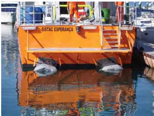
matches load capacity to fuel consumption at excellent speed. The load capacity is needed to carry all equipment and fuel on board. The vessel cruises at 11 knots consuming 185 l/h. The increased fuel efficiency allows it to spend more time at diving sites, with the waterjet propulsion system providing ultimate control for variable loads and sea condi-
