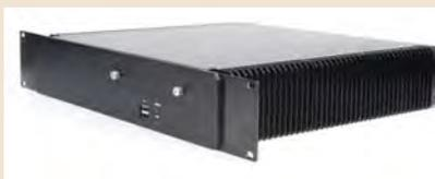
During 2010 Elektronix invested in development, design and quality assurance of a brand new range of marine approved PCs. Enix is based on a completely fanless design with Core 2 Duo CPU, and with several years of availability for all components. For standalone installation, wall mounting, or in 19" rack (2U och 3U). Industrial Wide-Temp Flash Disk (for a system with no moving parts), or 2.5" Industrial 24 / 7 hard drive.
