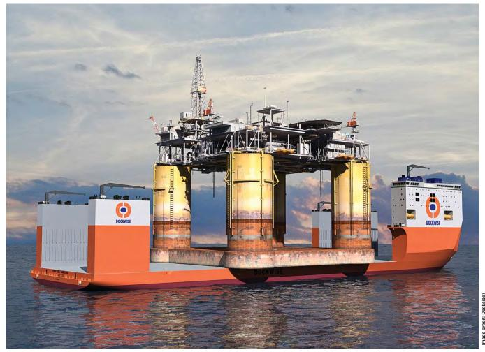
Dockside's new Super Vessel, Dockwise Vanguard presently under construction at HHI shipyard in Korea is due for completion in the latter part of 2012. It will have a capacity of more than 110,000 metric tons, and deck size of  $900 \times 230$  ft  $(275 \times 70 \text{ m})$ .
