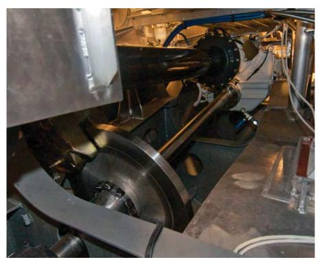
ZF Marine supplied the complete propulsion system, apart from the engines, including this ZF550 V-drive gear and shaft brake for the smaller C18 engine.
