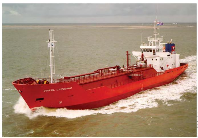
The 1,666-dwt, 262 ft. MV Coral Carbonic was built in 1999 for the transport of liquid CO2. The quality of the system ensures safe handling of the gas which can be used for human consumption and cannot be carried in other gas tankers.
