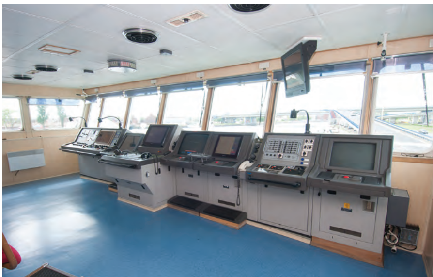
The expansive bridge of the Navigator XXI has extra radar monitors and chart tables for students.
